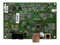
Photline MBC are a family of automatic bias controllers specially designed to lock the operating point of LiNbO<sub>3</sub> Mach-Zehnder modulators near the quadrature point and ensure a stable operation over time and environmental conditions.
